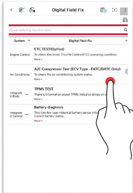
2. Check the basic description and test condition for the test, and touch 'OK' button.
