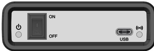
[Figure 1] Power switch of ADL body
