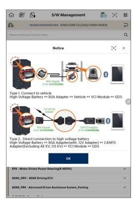
3. After checking the inspection purpose and conditions, press the 'OK' button.
