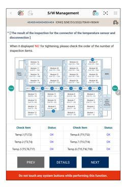
9. After final re-inspection of connector tightening presence/absence, the test result is displayed.
