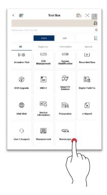
4. Attempt to connect USB automatically. Once USB connection is completed, the screen moves to the photo taking screen.
