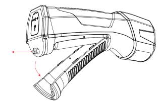
3. Take out the battery and replace it with a new battery.
