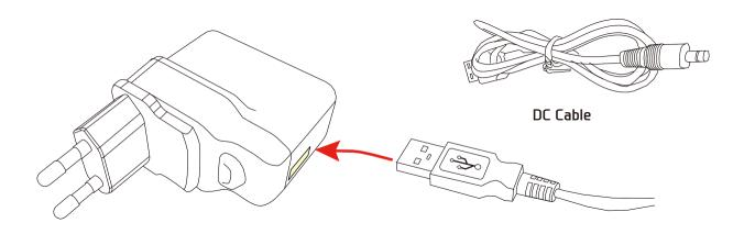
2. Peel of the waterproof cover on the rear side of the Main Body, and connect DC cable to DC input terminal.
