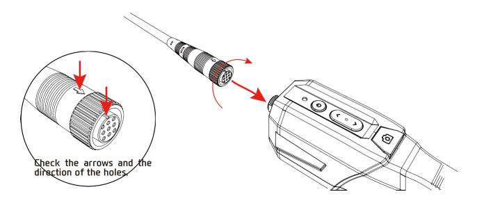
2. Mount the camera on the opposite side of the Flexible Tube, and fix it by rotating the screws.
