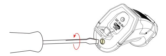
2. Take out the screw, and disassemble the batter cover on the handle side downwards.
