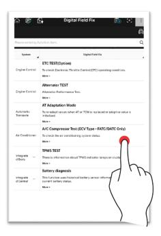
2. Check the basic description and test condition for the test, and touch 'OK' button. Proceed the next process by following the guidance for each function.
