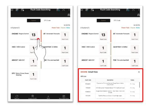
If you select a fault code in the detailed screen, it is switched to 'Fault Code' screen, which provides additional information.
