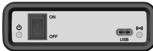
[Figure 1] Power Switch of ADL Main Body
