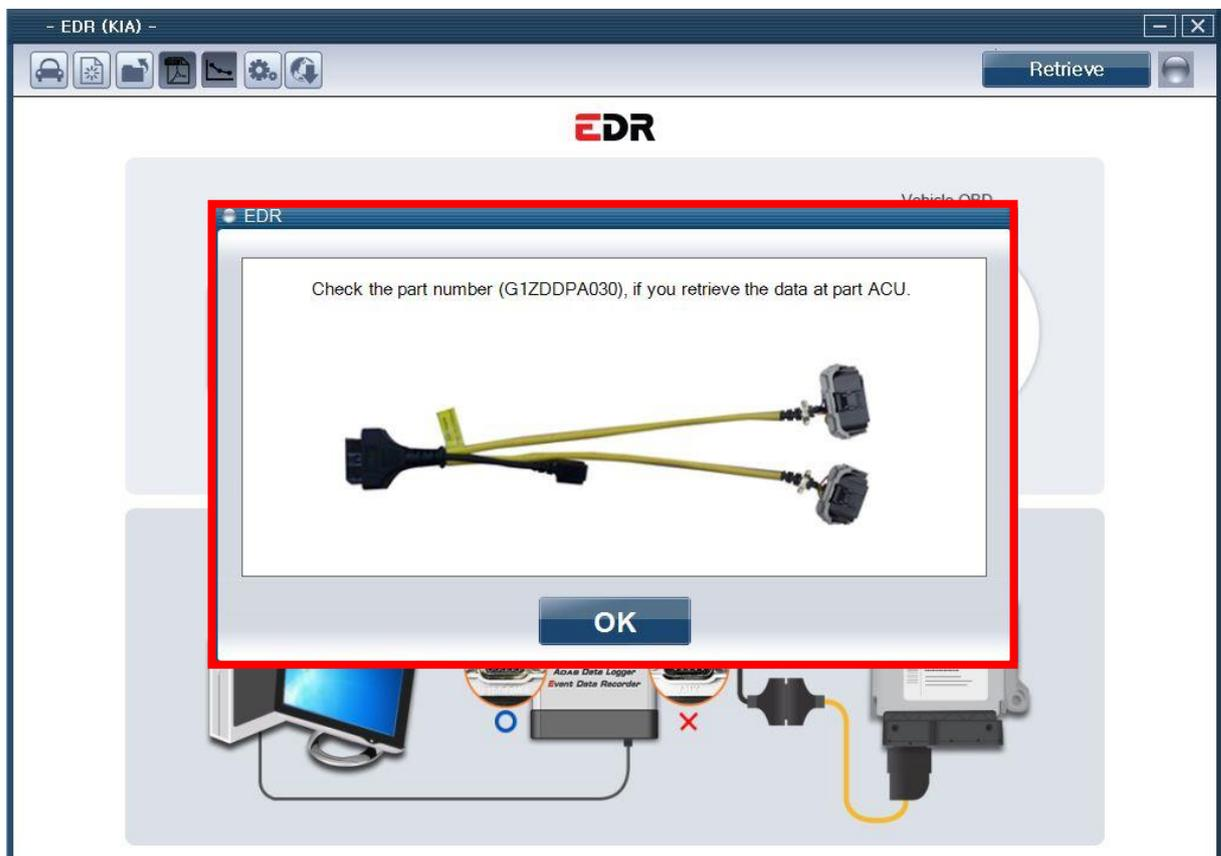
[Figure 5] ADL Connector Component Number Check
