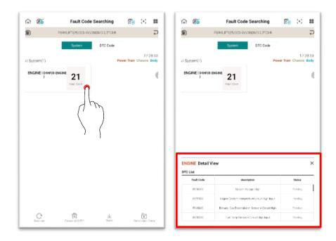
If you select a fault code in the detailed screen, it is switched to 'Fault Code' screen, which provides additional information.
