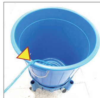
C. Set “Coolant discharge hose” to the drain bottle.
