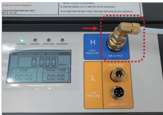
A. Install “Air Injection Adapter” to the “High Pressure Air Output” Port.
