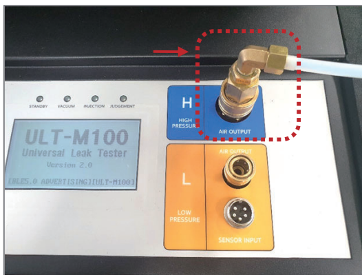
A. Install "Air Injection Adapter" to the "High Pressure Air Output" Port.
