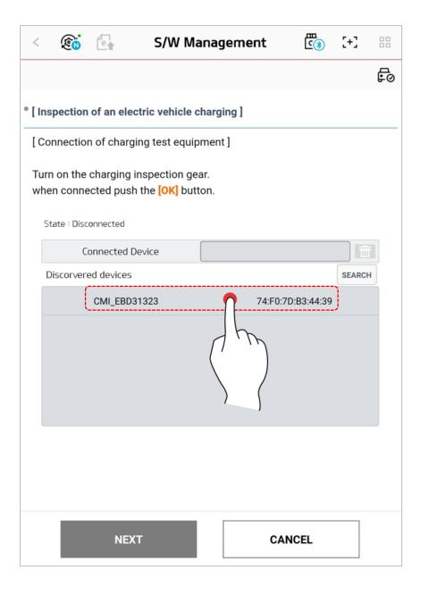
After the selected, the equipment is registered in "Connected Device" list, tab button at the bottom of the screen.
