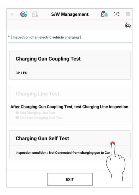
Once you enter into the function screen, the self-test will begin, and the results will be shown on the screen after approximately 20 seconds.
